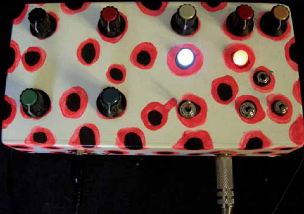
6-Bit Noise Generator
